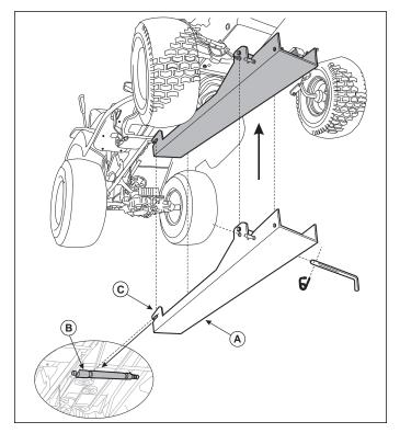
Figure 8. Hitch Installation
